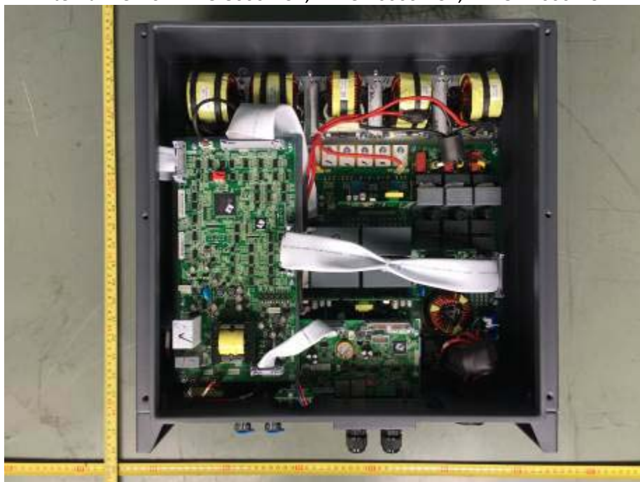
Internal view of EVVO 3000TL3P, EVVO 4000TL3P, EVVO 4800TL3P, EVVO 5000TL3P, EVVO 6000TL3P
