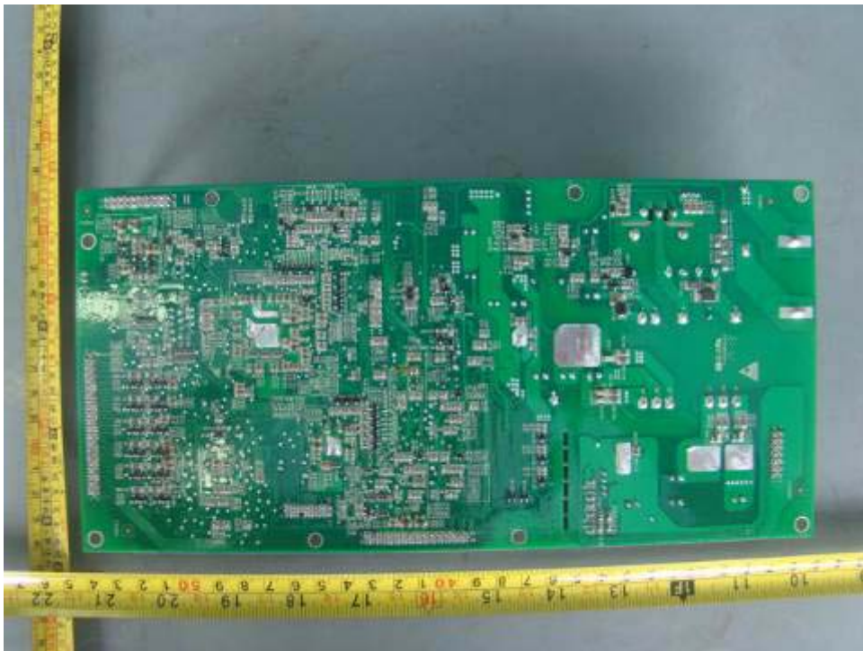
Trace side of control board
